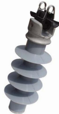
Designed for medium voltage networks up to 24kV. Insulator is made of hot-dip galvanized steel, aluminum alloy and two-component polymer. Designed to restrain corrosion and environmental conditions. Implemented seesaw on insulator enables usage on various terrain and gives possibility for angle variation up to 45°. It is designed in accordance to the standard IEC 61109.
